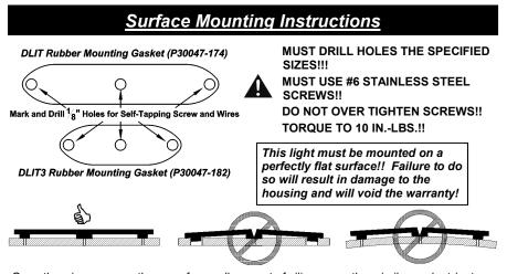
Once the wires are run, the use of a small amount of silicone or other similar sealant (not included) is recommended to seal the wire hole and prevent your wires from becoming damaged.
